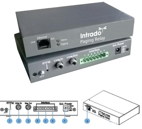
RTFM Button - When pressed momentarily the Relay will announce it's ip address via the line-out ports / when held for 30 seconds the Paging Relay will default back to factory settings
